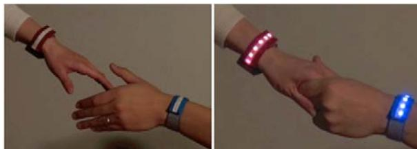
**Figure 1: Enhanced Touch: Sensing touches and identifying others can be done by the wearable device with electrodes.**
