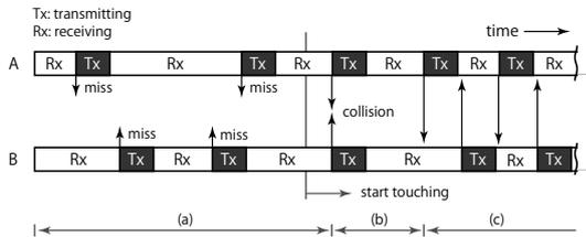
Figure 3: Procedure of communication between two developed devices.
